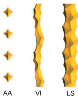
Figure 2. Void volumes of the crystal structures of AA, VI, and LS that can hold a spherical “probe” with a diameter of 2.6 Å.
